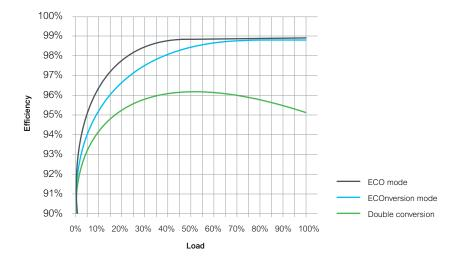
Efficiency curves based on 1000kW, 415V UPS data.
